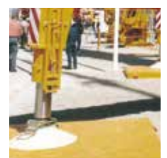
LINNOTAM float pads Ø 700 mm on a truck crane
