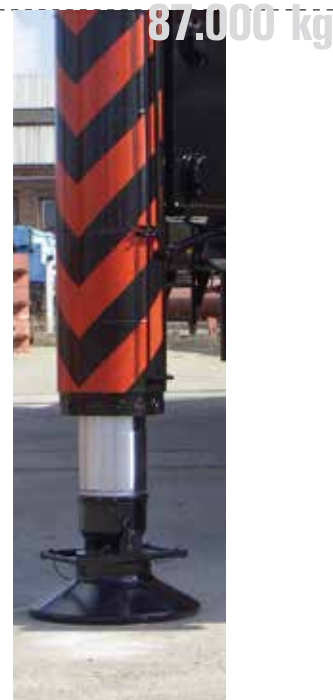
LINNOTAM float pads Ø 400 mm on a railway crane
